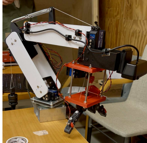
(b) Redesigned robotic arm with updated joints, tendons, and end-effector.
